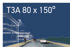
T3A 80 x 150° Application: Asymmetric light distribution for Residential street.
