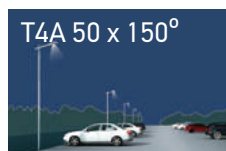
T4A 50 x 150° Application: Asymmetric light distribution for wide area.
